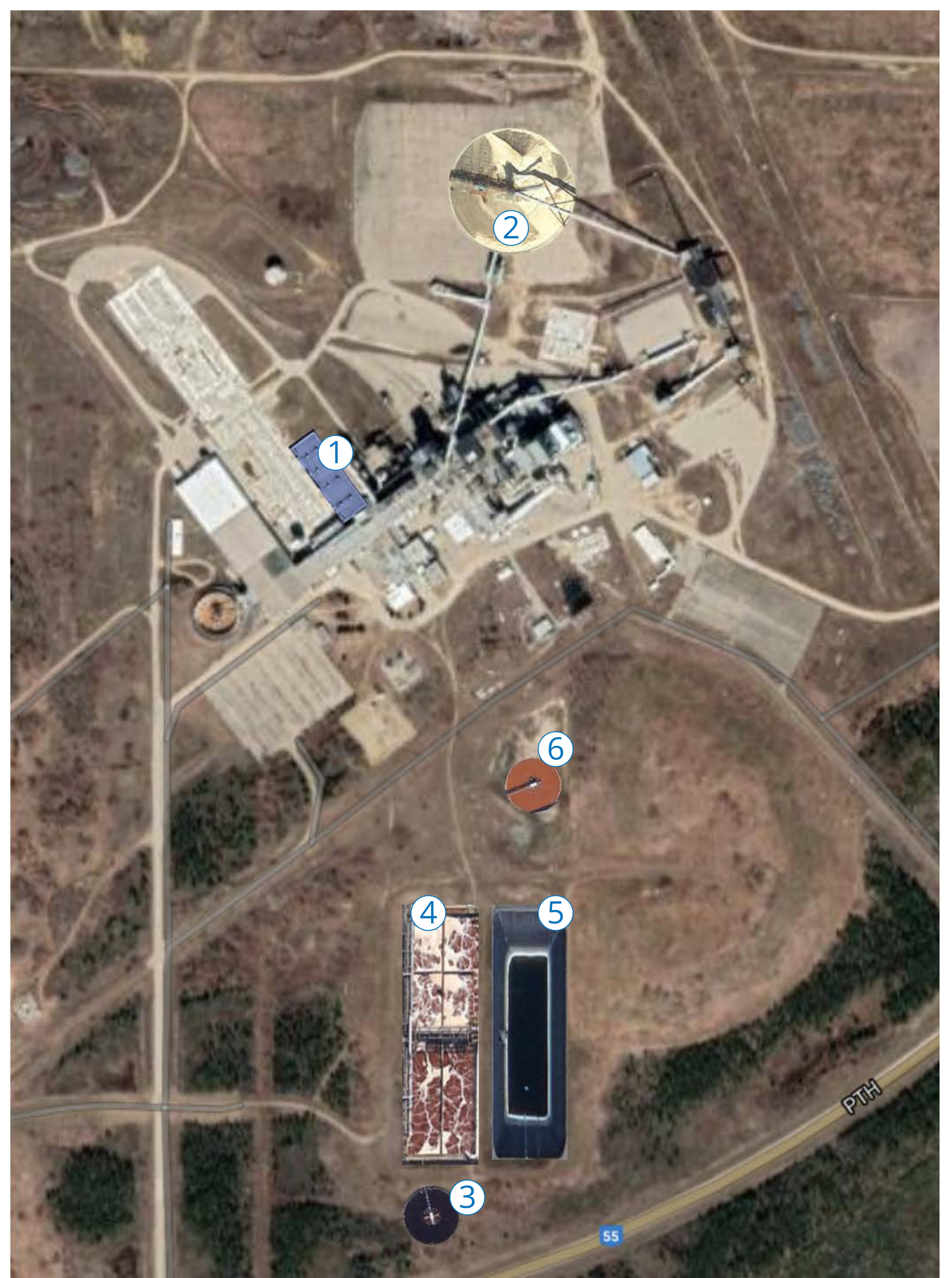
Photo above: Six construction sites outside the legacy mill footprint: 1. Fibreline building; 2. Wood chip stacker reclaimer; 3. Secondary clarifier; 4. Activated treatment basin; 5. Diversion basin; 6. Primary clarifier.
